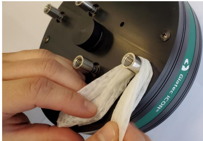
Representation of cleaning the iCOR shafts
