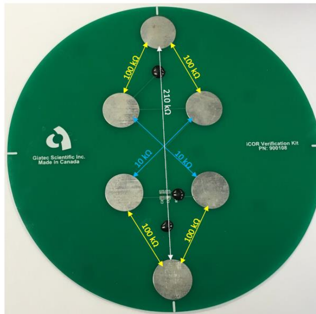
Schematic demonstration of the continuity on the verification disk
