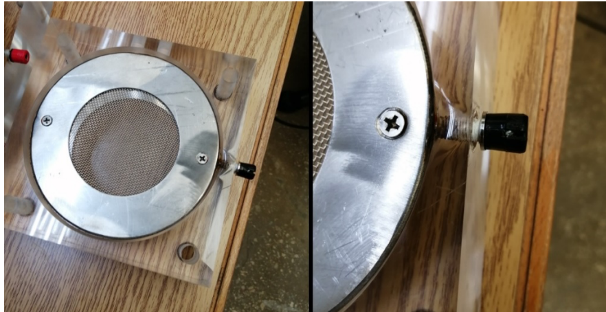
Example of corrosion on the metal faceplate due to lack of contact with the connector
