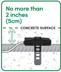
Install the transmitter on rebar no more than 2 inches (5cm) from concrete surface
