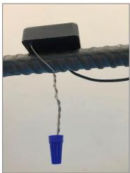
Additionally, electrical tape or zip ties are required as per usual to fully secure the sensor against rotation around rebar.
